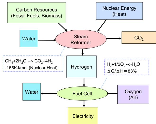
**Fig.4 Concept of Synergistic Electricity Generation Using Carbon Resources and Nuclear Energy**
