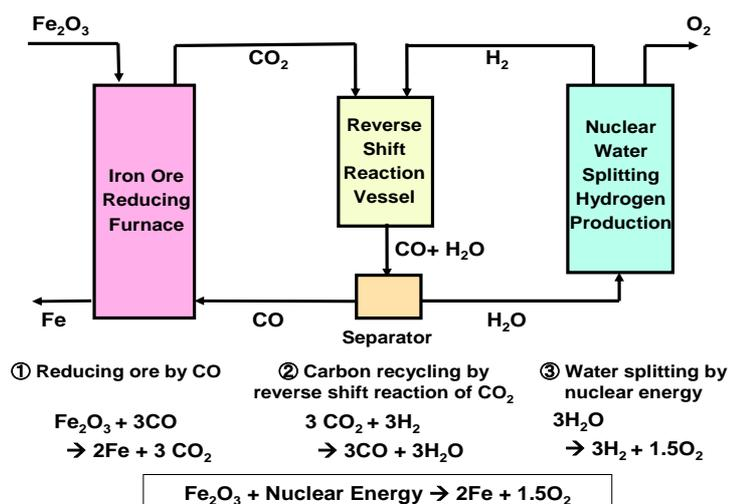
**Fig.3 Concept of Nuclear Iron Making by Carbon Recycle**
