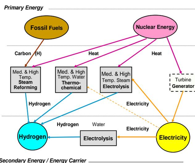
**Fig.1 Methods for Hydrogen Production by Nuclear Energy**
