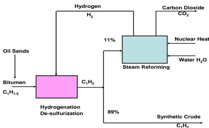
Fig.2 Nuclear Upgrading of Oil Sands Bitumen to Synthetic Crude Oil
