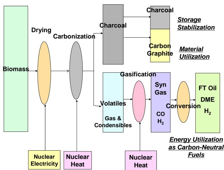
**Fig.6 Concept of Nuclear Biomass Carbonization and Gasification**
