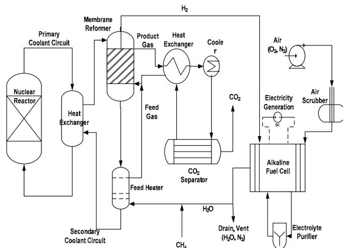
**Fig.5 Application of Synergistic Electric Generation Using Natural Gas and Sodium Cooled Reactor**
